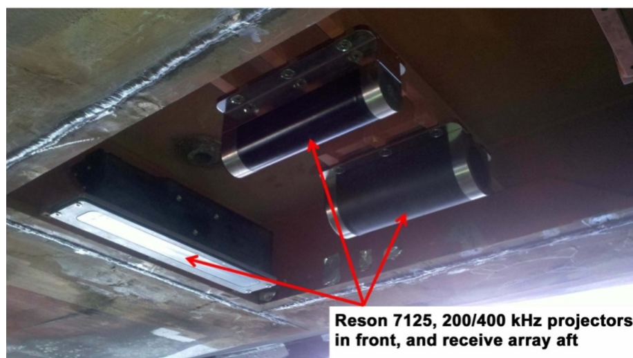
Figure 2-3. Picture of the hull-mounted Reson 7125 transmit/receive array.
