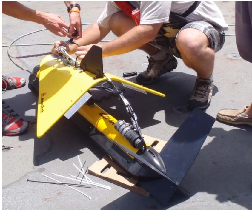
Figure 2-4. Picture of the Edgetech towfish used to collect sidescan sonar data.
